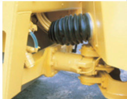
The bolt-on oscillating, articulation joint is designed for long life even in tough site conditions
