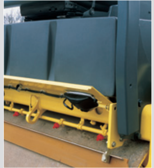
Wind protected spray nozzles provide even drum coverage
